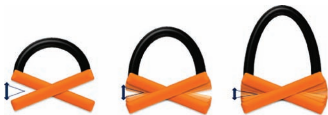
Figure 1. Schematic representation of strapped atropo-enantiomeric PBIs and variation of the naphthalene units twisting angle depending on the bridge length.
